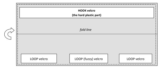
Fold the sleeve in half so that the hook and loop velcro are sealed together. Press along the fold line
